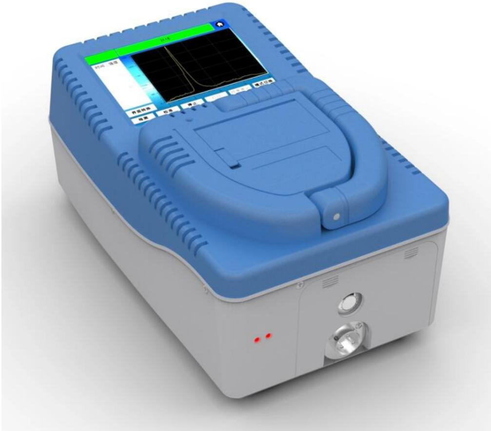
Securina SD300A portable explosive and narcotics trace detector is a narcotics and explosives detection device. Based on the principle of ion mobility spectrometry, it can accurately detect particles or vapor of trace amounts of explosives and narcotics, and give the ingredient names.
