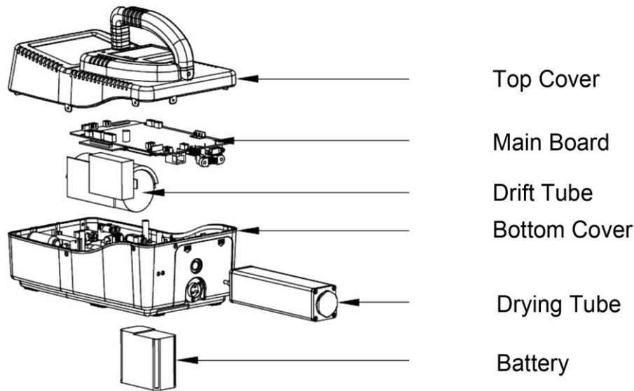
1. The drift tube: It is the core component of SD300A, where samples can be tested.
